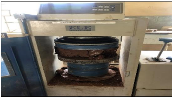
Plate 5: Compressive strength testing of bricks
