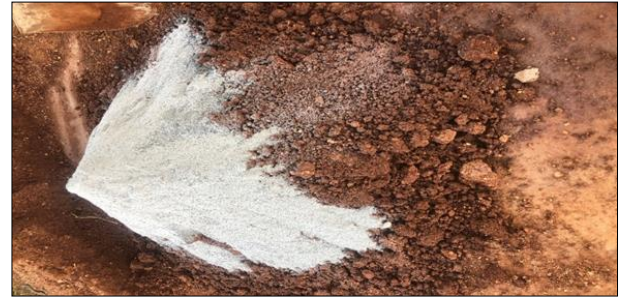
Plate 2: GSA and Laterite soil before mixing.
