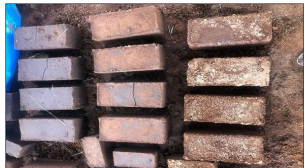
Plate 4: Bricks during curing
