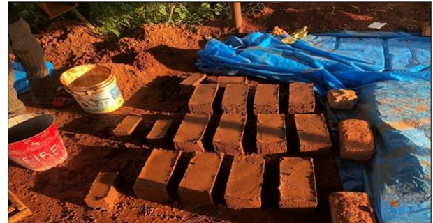
Plate 3: Molded bricks before curing
