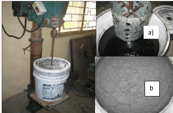
Plate 2: Flootation unit set-up; (a) coal slurry with percentage cleaning agent before and (b) after stirring.
