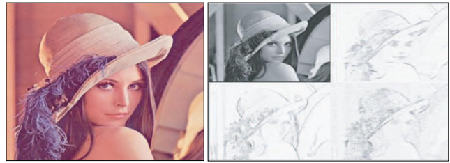
Fig 2: Wavelet Decomposition of an Image Component. The image has been modified: the average detail has been lightened and the horizontal, vertical and diagonal details are shown as negative images with a reversal of white and black, because of constraints of the printing process.
