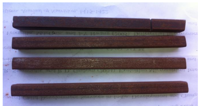
Fig 2.3: mild steel samples after 35 days of exposure
